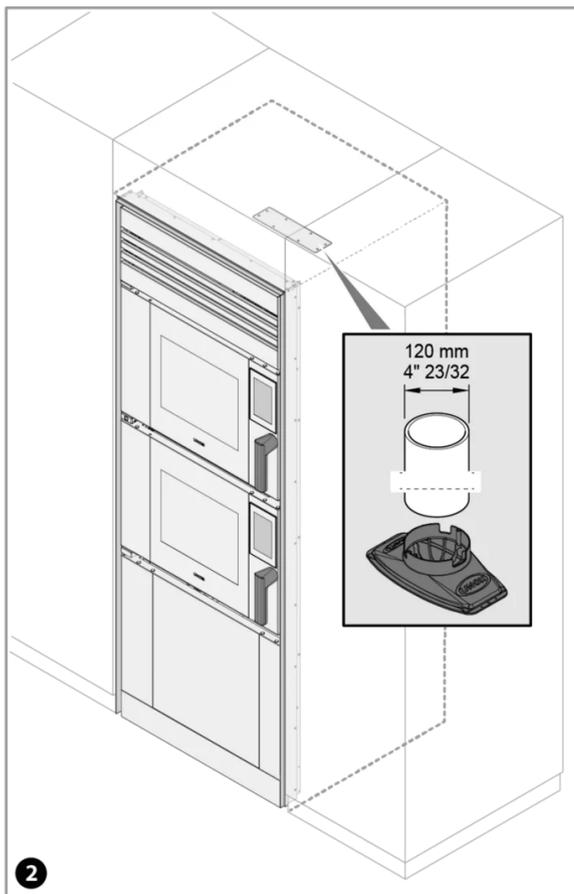
**Option 2 - Non-flush installation with XUC501 steel frame**
